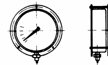
5. circular gauge for flush-mounting, with rear rim and front ring B, 100, 160 mm dia.
