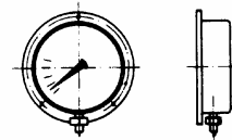
2. circular gauge for surface-mounting 100, 160 mm dia.
