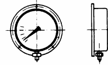
1. circular gauge, 100, 160 mm dia. as standard
