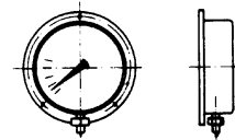
2. circular gauge for surface-mounting, Ø100 mm, Ø160 mm,
