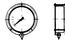
5. circular gauge for flush-mounting, with rear rim and front ring B, Ø100, Ø160 mm
